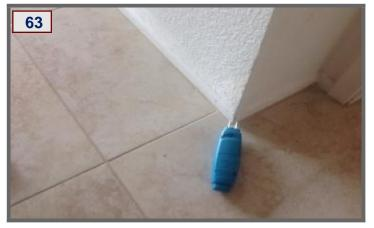
Kitchen in Wall Moisture Noted With Moister Probe , Kitchen in Wall Moisture Noted With Moister Probe
